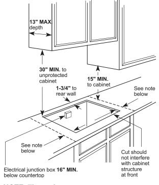
NOTE: This cooktop has been approved for 0" spacing to adjacent surfaces above the cooktop. However, a 6" minimum spacing to surfaces less than 15" above the cooktop is recommended to reduce the exposure to steam, grease spatter and heat.
