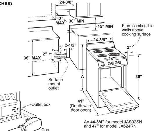
Recommended acceptable electrical outlet area. Orient the electrical receptacle so the length is parallel to the floor.
